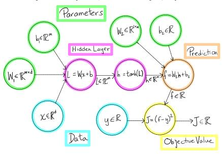
The crucial new piece here is the nonlinear **hidden layer**, which is what makes the multilayer perceptron a significantly larger hypothesis space than linear prediction functions.
