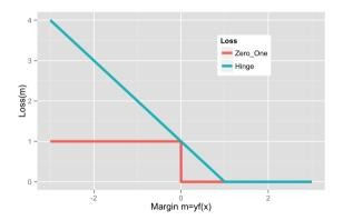
Hinge is a convex, upper bound on 0-1 loss. Not differentiable at m=1.
