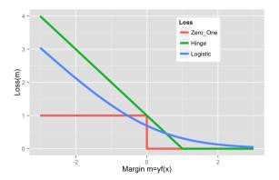
Logistic loss is differentiable. Logistic loss always rewards a larger margin (the loss is never 0).
